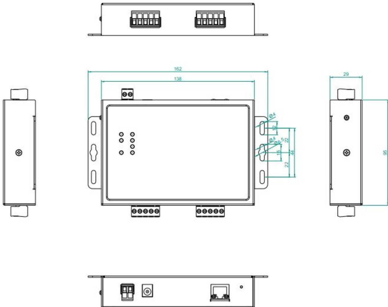
Din-rail mounting (unit: mm)
